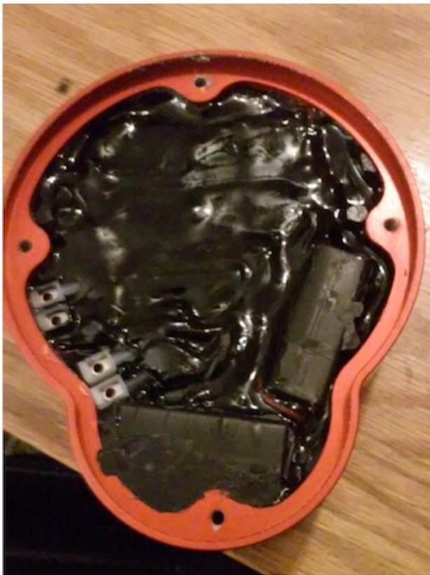
The O-Cube as Frank received it, with back of the housing removed. Filled with mastic.
