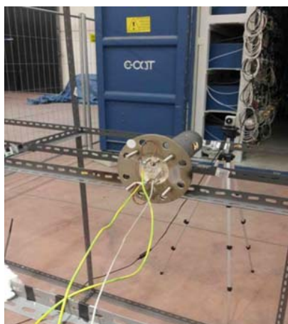
Fig. 2. The E-Cat HT2 used for the March test. The device appears as a steel cylinder, 9 cm in diameter, and 33 cm in length, with a steel circular flange at one end 20 cm in diameter and 1 cm thick.
