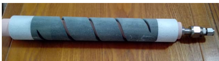
Figure 31. The assembly of the corundum vessel and silicon carbide heater.
