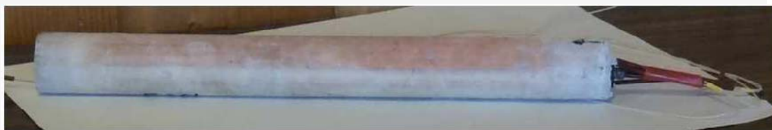
Figure 20. The heater with the thermal cell installed inside
