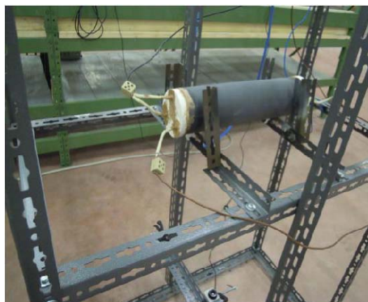
Fig. 1. E-Cat HT on support frame. The power cables to the internal resistor coils are visible, as well as the IR camera in the lower part of the photograph.
