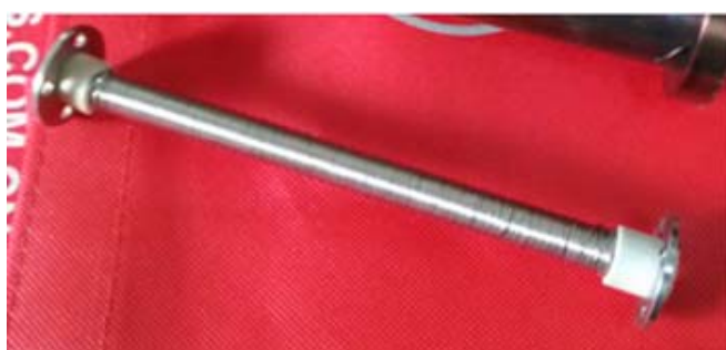
Figure 16. The nickel wire wound on the stainless-steel tube.
